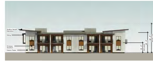
9 Building E - North Elevation 1/16" = 1'-0"
