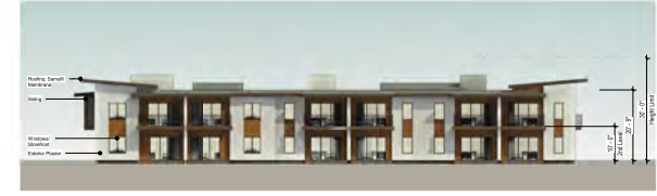
4 Building D - North Elevation 1/16" = 1'-0"
