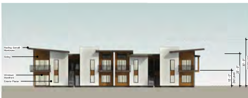
10 Building E - South Elevation 1/16" = 1'-0"
