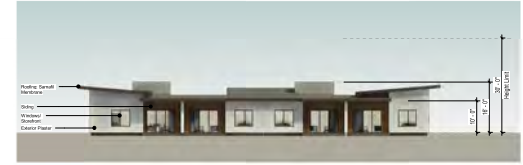
4 Building F - North Elevation 1/16" = 1'-0"
