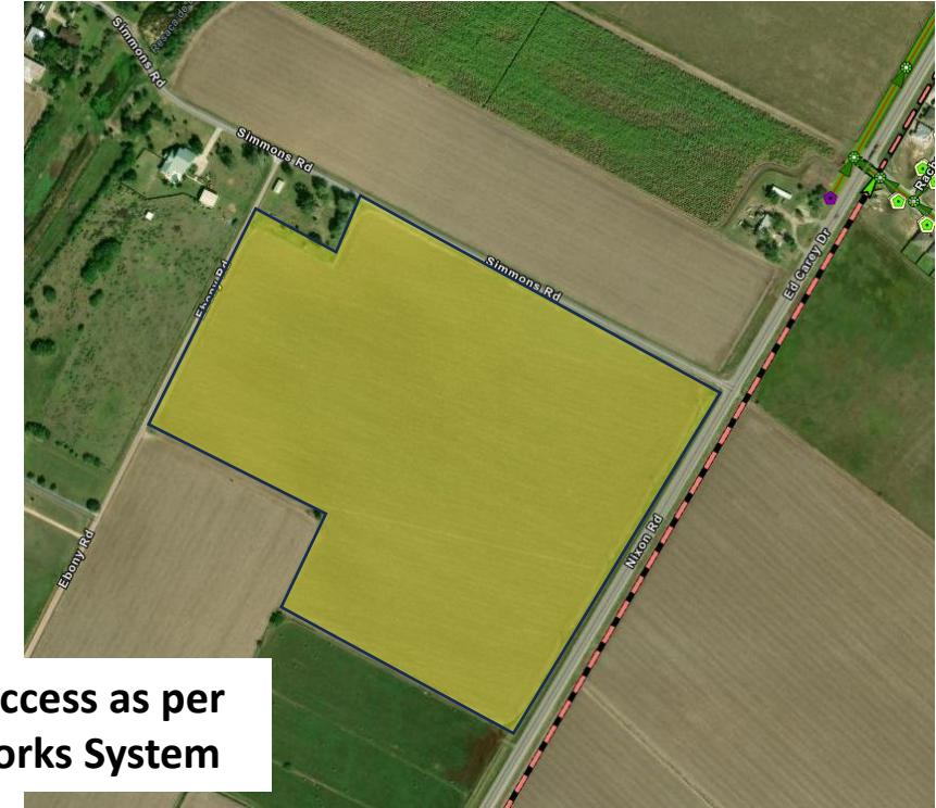
Regarding sewer infrastructure, there is an existing 6" PVC San. Sewer force main that follows along the east side of Ed. Carey. There is an existing 15" San. Sewer gravity main that is found near 720 LF from the property. The gravity main is around 7.5" ft deep. This may not be deep enough to serve the property. As such, a sanitary sewer lift station may be required with a FM that discharges into the existing gravity system.
