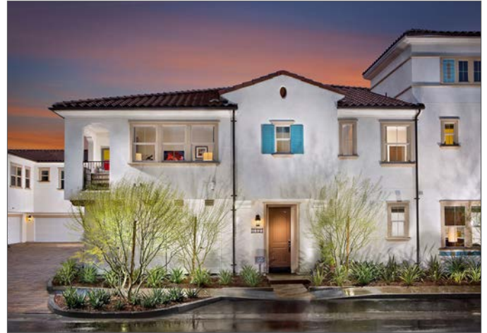
The mass of this multi-family building is broken up with a gable that extends above the roof line and marks the entry into the unit.
