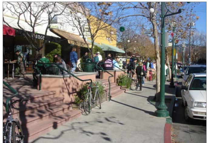
Door Yard Example - outdoor seating areas raised above the adjacent sidewalk and accessed by stairs. A low wall above the terrace level provides a place to sit.
