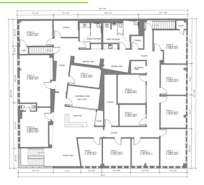
SECOND FLOOR PLAN AS-BUILT SCALE 1/4" = 1'-0"
