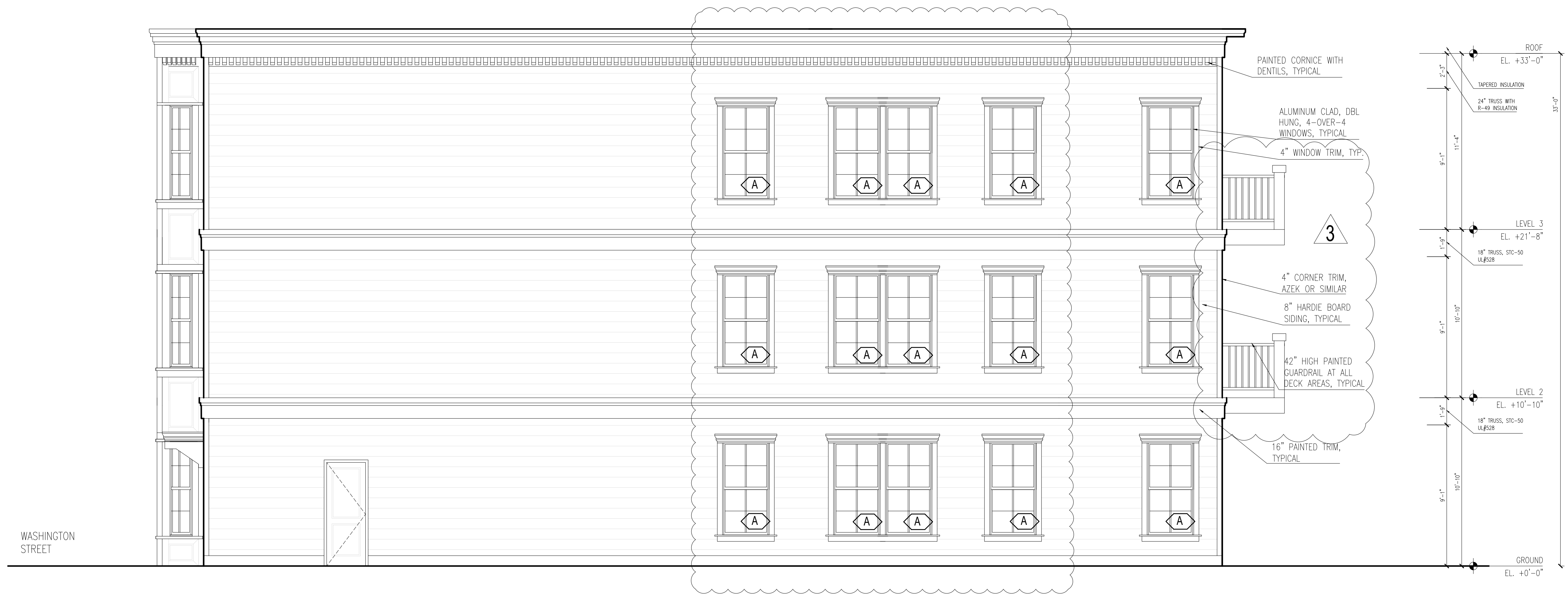
3 PROPOSED RIGHT SIDE ELEVATION SCALE: 1/4" = 1'-0"
