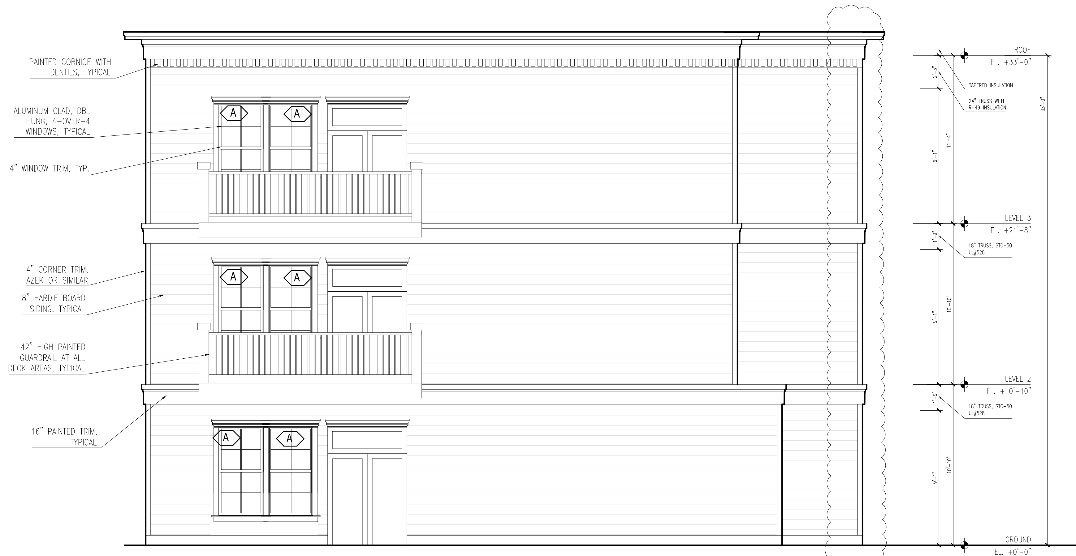
2 PROPOSED REAR ELEVATION SCALE: 1/4" = 1'-0"
