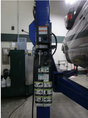
Photo #7 View of above ground hydraulic lift located in the shop.
