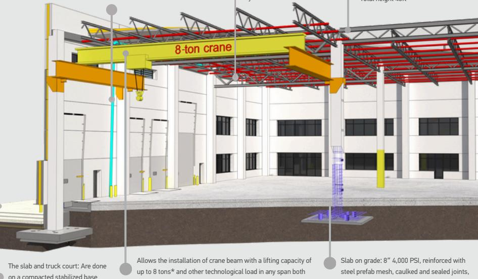
Bottom: Prefabricated 3-layered precast concrete insulated panels, R-value 16, painted: int - white, ext - according to customer's request
