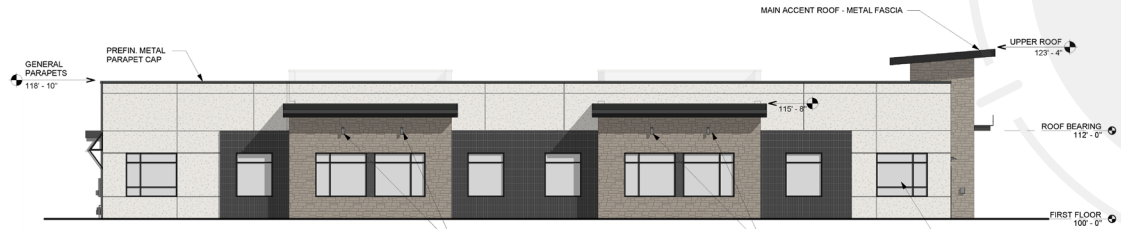
2 PLANNING ELEVATION - EAST SCALE: 1/8" = 1'-0"
