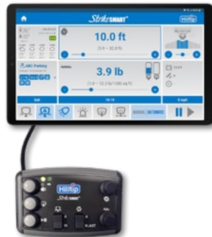
8,7" touch screen and control panel
