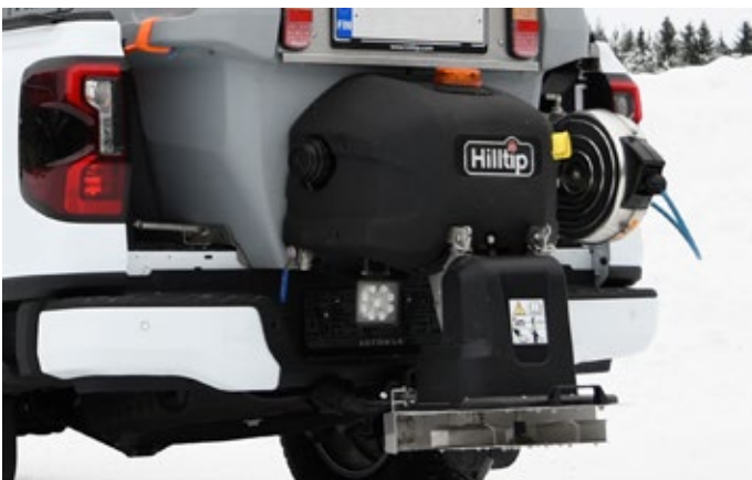
Beacon light (orange) & LED work light (white)
