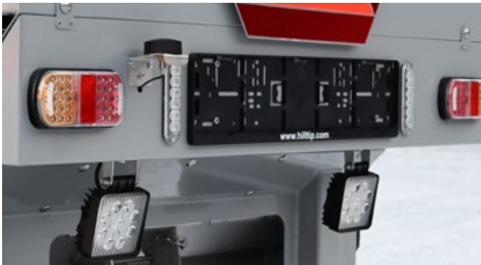
Lighting kit: 2 LED work lights, 2 strobe lights, and 2 LED stop/tail/brake lights
