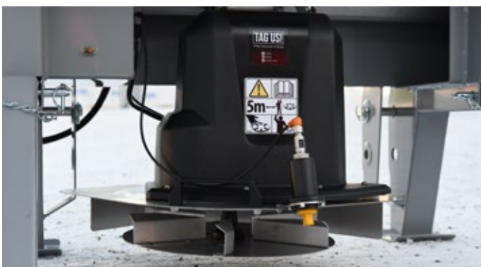
End of material alarm sensor on spinner
