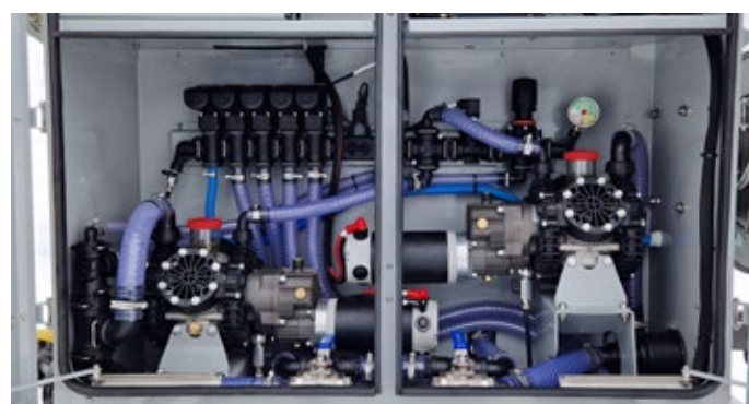
Self-priming hi-pressure & flow Diaphragm pumps, motors and valves in closed cabinet
