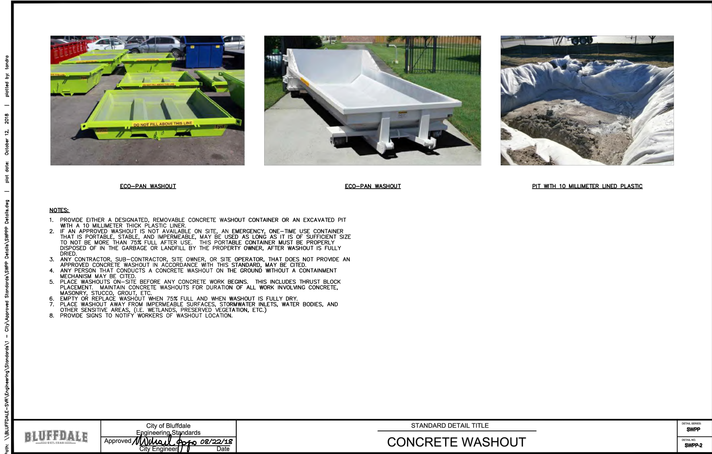
CONCRETE WASTE MANAGEMENT 1 SCALE: NTS
