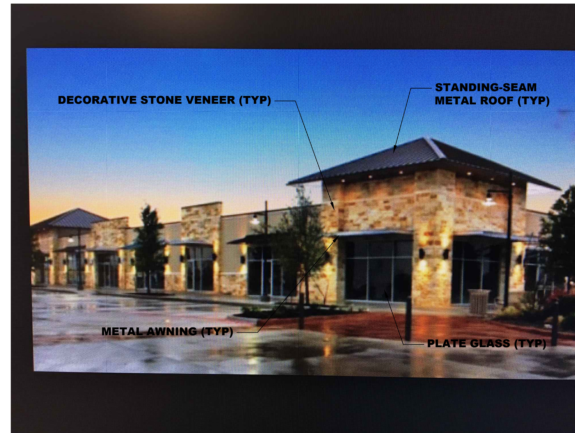
RETAIL BUILDING ELEVATION "C" NTS
