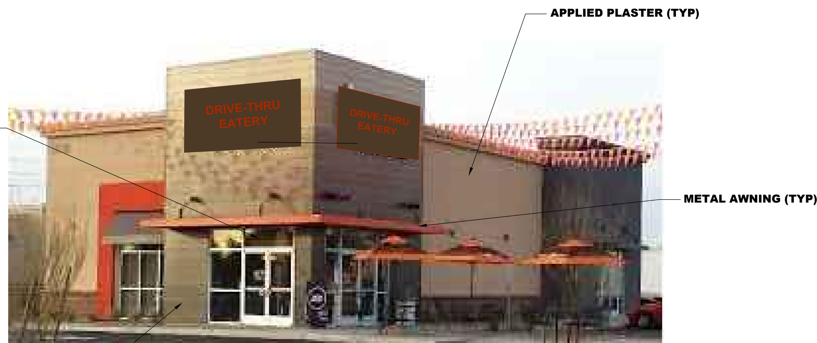
DRIVE-THRU EATERY BUILDING ELEVATION "A" NTS
