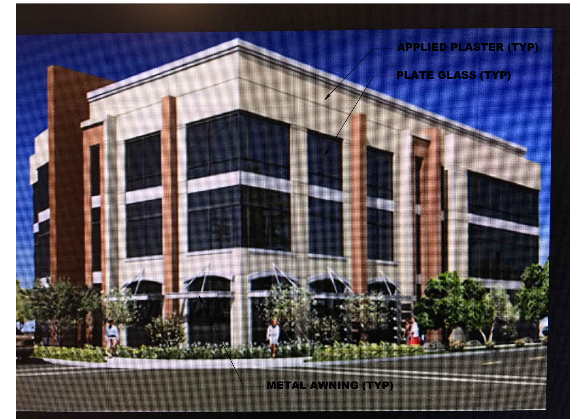
MEDICAL BUILDING ELEVATION "B" NTS
