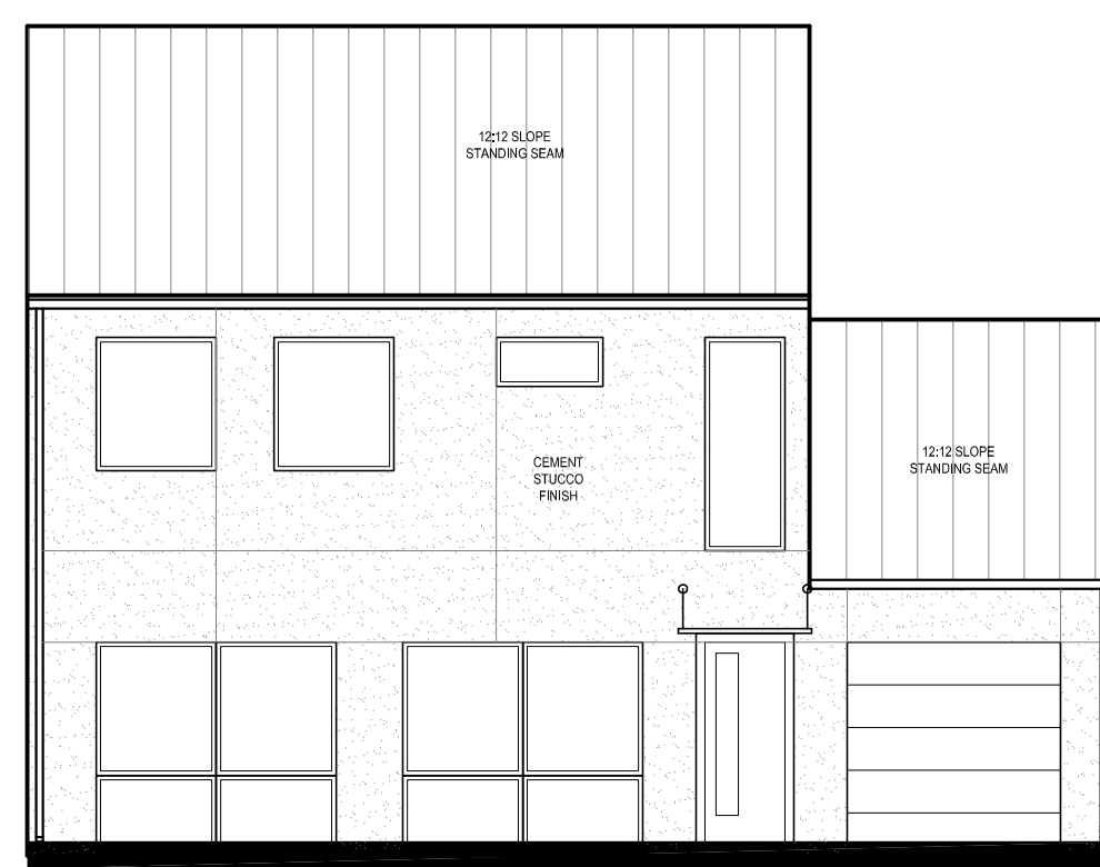
ADU South Elevation 01 1/4" = 1'-0" Re: A.001
