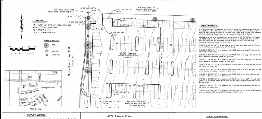
Bearings are based on the U.S. State Plane Coordinate System (NAD83) Texas North Zone.
