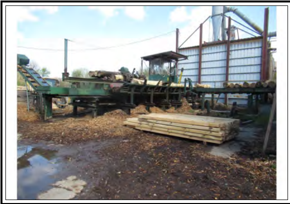
Log infeed to mill showing bark conveyor and side view of sawdust storage building
