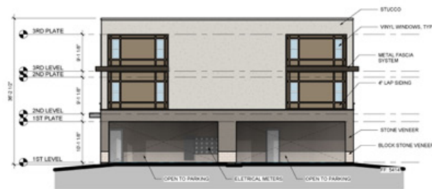
3 BUILDING 1-RIGHT SIDE ELEVATION (PRIVATE ALLEY) 3/32" = 1'-0"
