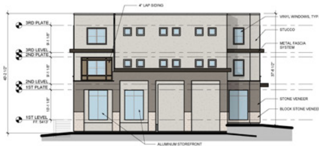
2 BUILDING 1-LEFT SIDE ELEVATION (W. 93RD PL.) 3/32" = 1'-0"
