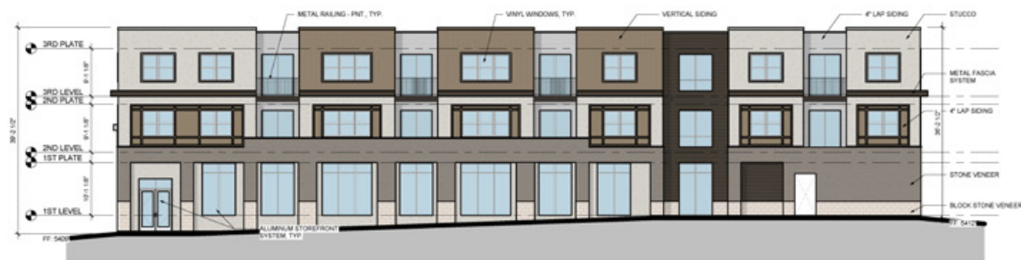
1 BLDG 2-REAR ELEVATION (MCINTYRE ST.) 3/32" = 1'-0"
