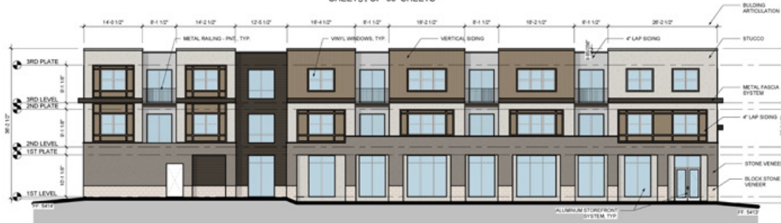
4 BUILDING 1-REAR ELEVATION (McINTYRE ST.) 3/32" = 1'-0"
