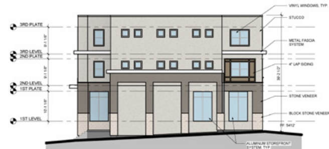
2 BLDG 2-RIGHT ELEVATION (W. 93RD PL.) 3/32" = 1'-0"
