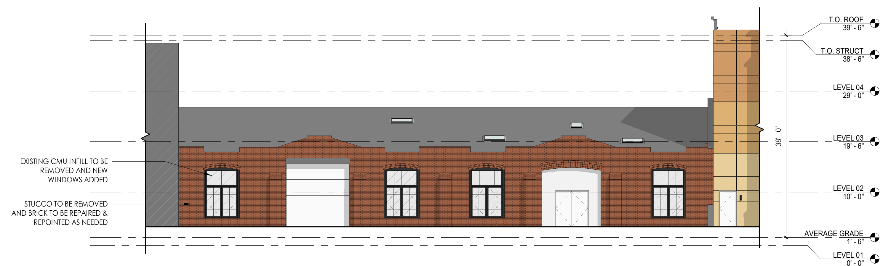
1 | MANNING ST ELEVATION - EXISTING SD005 | 3/32" = 1'-0"
