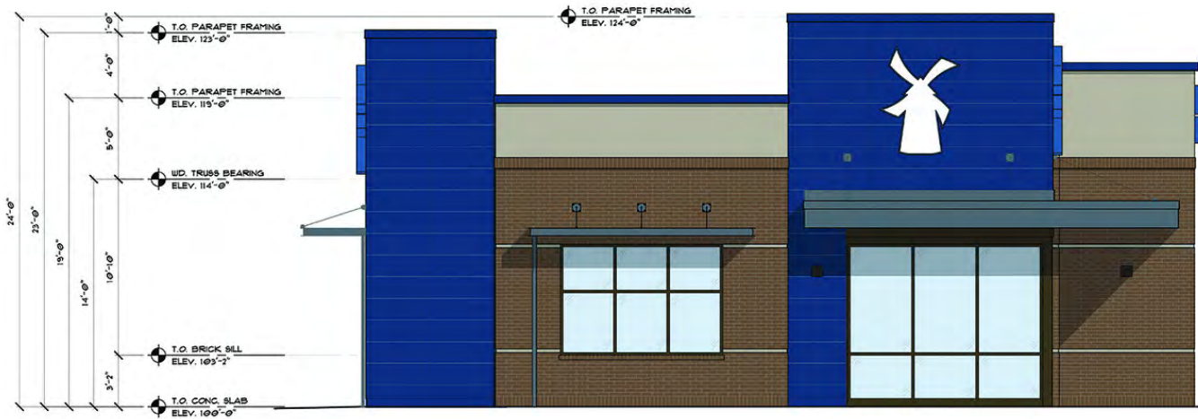
2 SOUTH ELEVATION (ALLEY) 1/4" = 1'-0"
