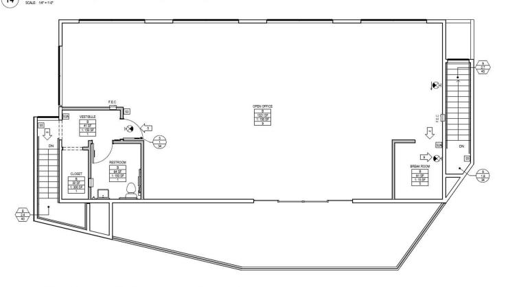
(16) SECOND LEVEL CODE AND OCCUPANT EXITING PLAN
