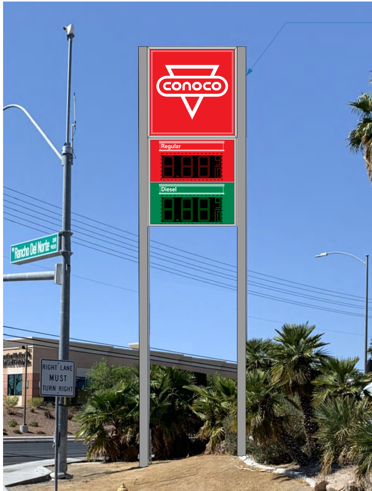
EXISTING PYLON w/ NEW FACES & LED PRICE CHANGERS SCALE: 3/16" = 1'
