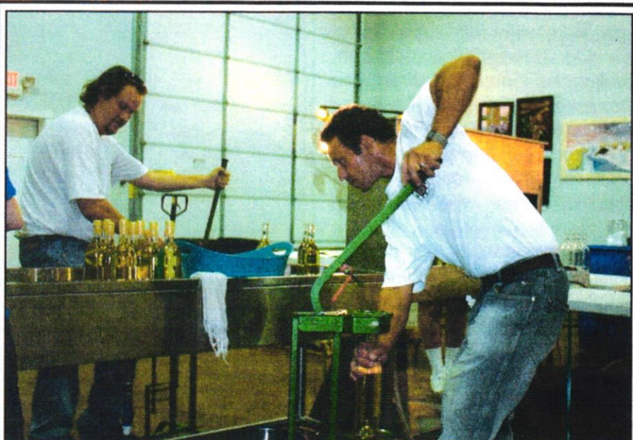
Two workers use leverage to insert corks into the recently filled bottles of wine. With both corking the bottles at the same time, the process is faster with only the foil seal and label left to do.
