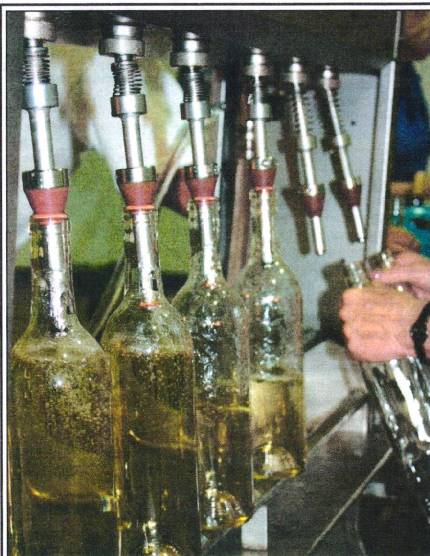
Workers hook up empty bottles to a machine that then fills them with a certain amount of finished wine. The bottles are then sealed and labeled for storage and sale.
