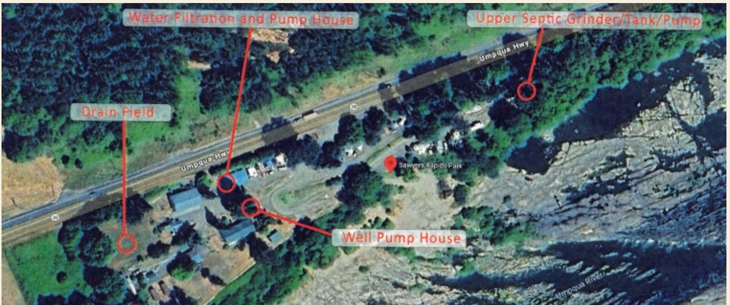
Aerial infrastructure diagram — water filtration, well pump house, septic systems, and drain field locations
