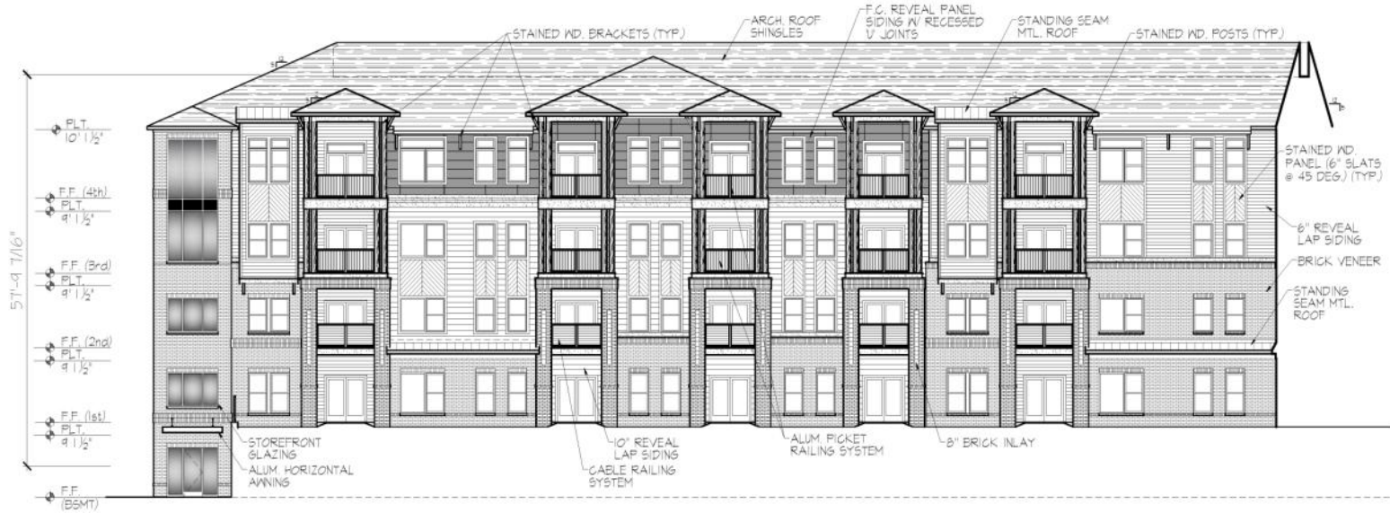
BLDG. A- FRONT ELEVATION (PARTIAL) SCALE: 1/8" = 1'-0"
