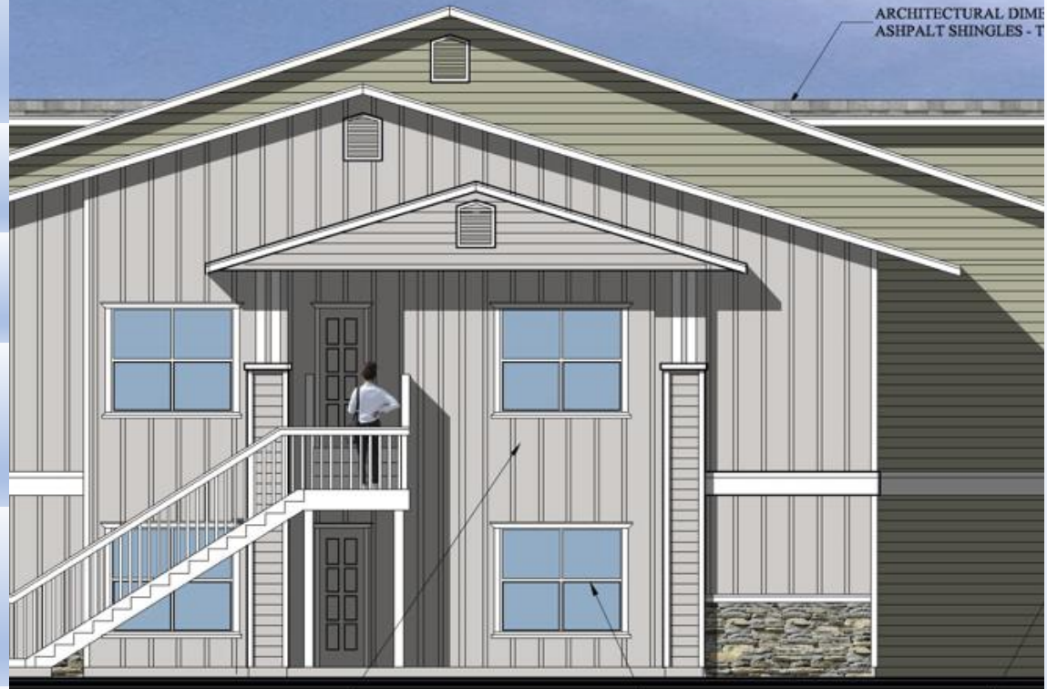
BOARD & BATTEN SIDING - PAINTED TYP
