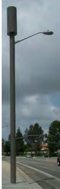
Example of Stealth Pole
