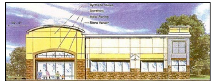
BUILDING 'J' NORTH EAST ELEVATION
