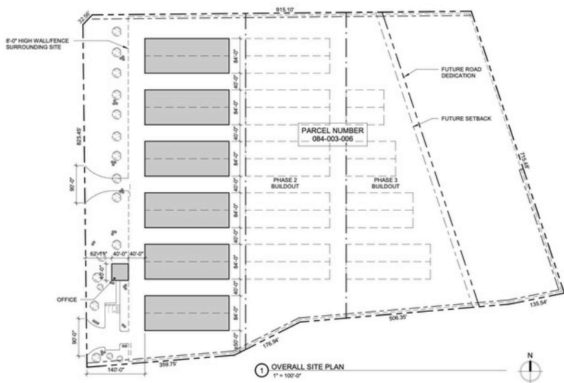
RED ARCHITECTS PROPOSED SITE PLAN LITT ROAD - RV & BOAT STORAGE
