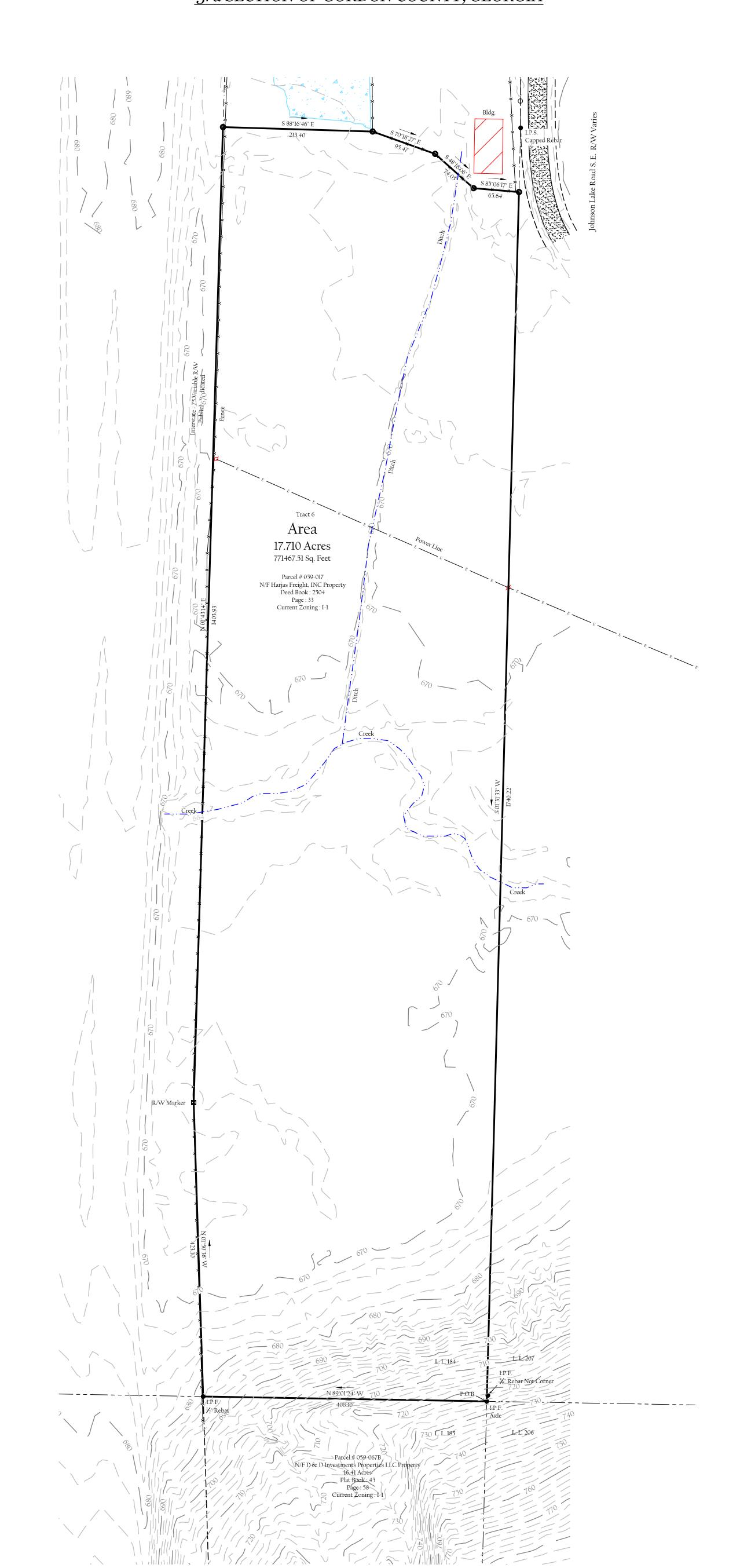
—LEGEND— I.P.F. = IRON PIN FOUND I.P.S. = IRON PIN SET R/W = RIGHT OF WAY P/L = PROPERTY LINE L.L. = LAND LOT LINE ø = POWER POLE € = CENTER LINE — X — X — FENCE LINE CONC. R/W MARKER
