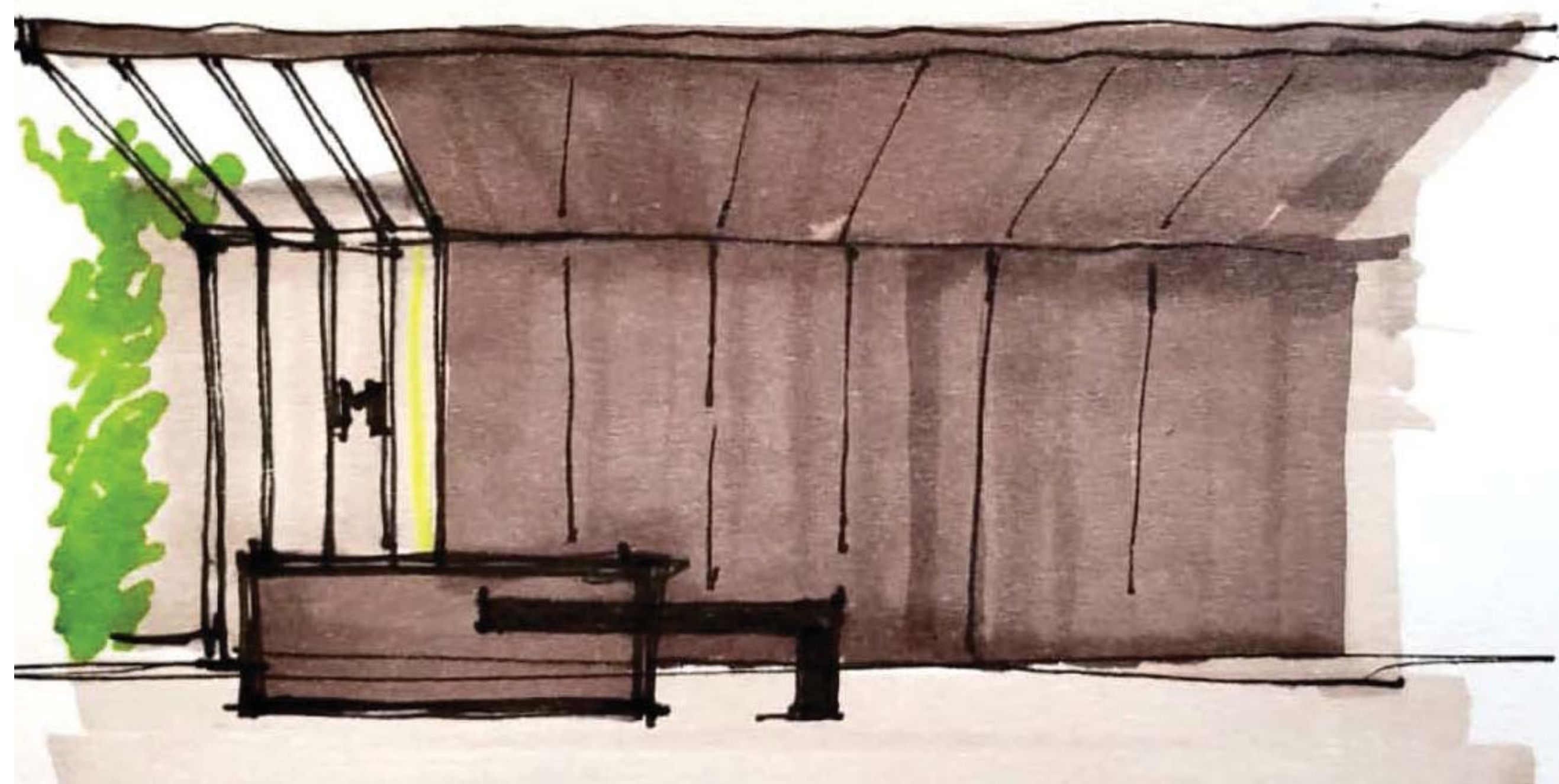
SOFFIT @ RECEPTION AREA: CEMENT WOOD BOARD & METALWORK
