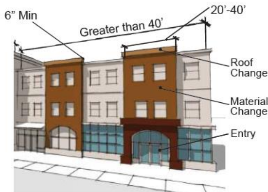
Figure 17.134-11: Building Facade Form Variation
