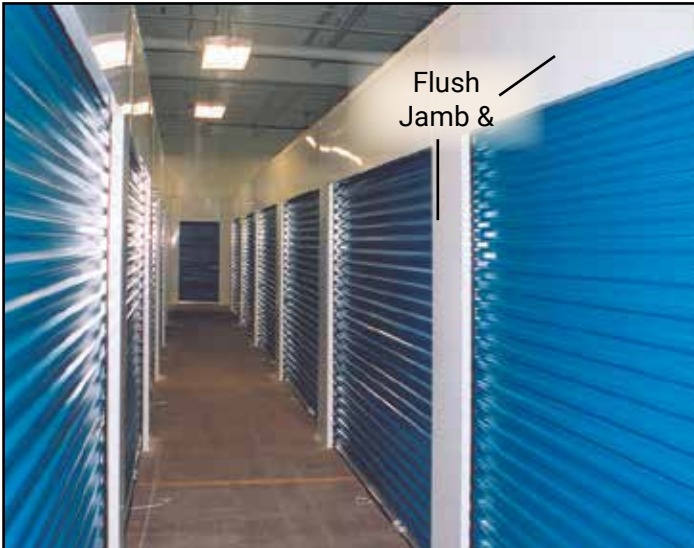
1a. The system consists of a door opening with bright white finish flush jambs and headers. Trachte's standard conversion system comes in heights between 7' & 10' in 6" increments. Special heights may be accommodated.
