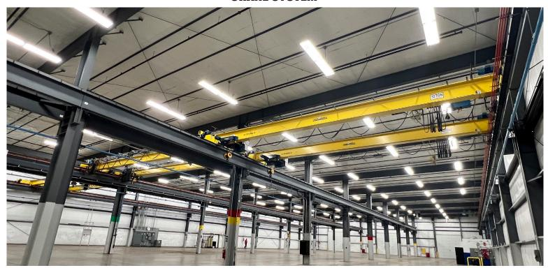
Building includes four 10-ton crane rails and two 5-ton rails. Top running cranes are commonly used for machine shops, warehouses, steel and metal fabricators, and heavy equipment maintenance facilities. Cranes are great for saving valuable floor space and cover a large work area.
