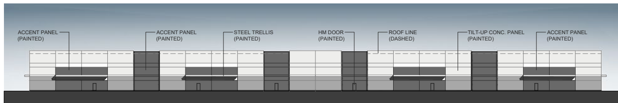
South Elevation (I-80)
