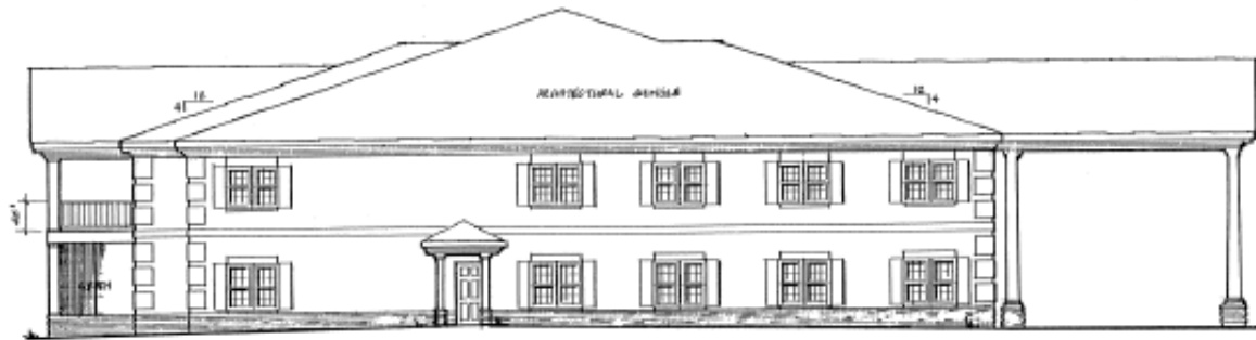
NORTH ELEVATION 1/8" = 1'-0" SOUTH ELEVATION SIMILAR
