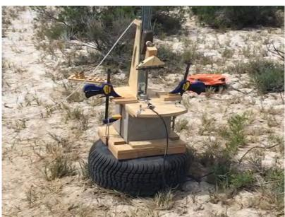
Figure 14: "Betsy Gun" apparatus used as a source for the seismic array.
