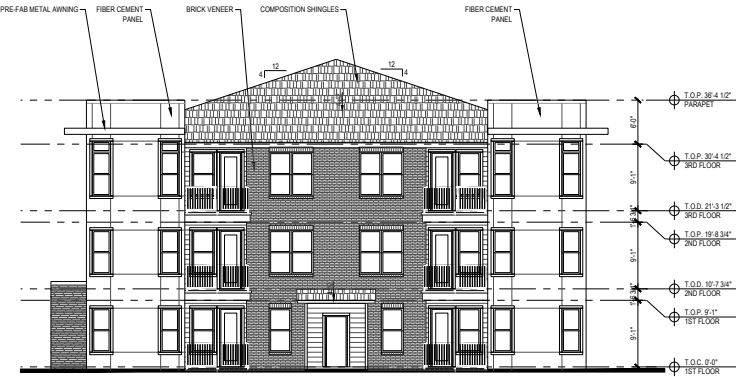
2 BLDG. TYPE I - SIDE ELEVATION SCALE: 1/8" = 1'-0"
