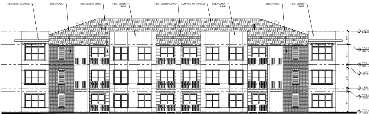
3 BLDG. TYPE I - REAR ELEVATION SCALE: 1/8" = 1'-0"
