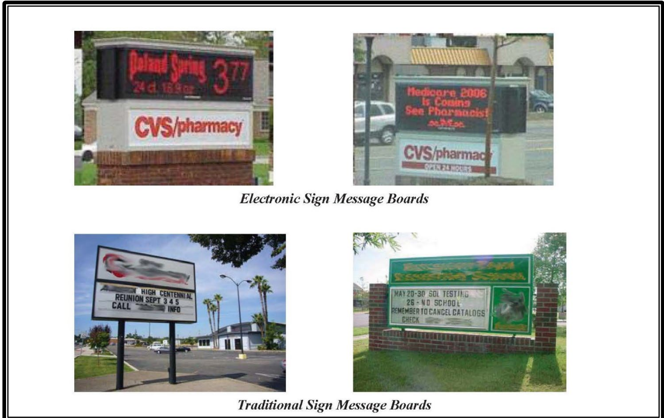
Figure VII-45 Sign Components – Sign Message Board
