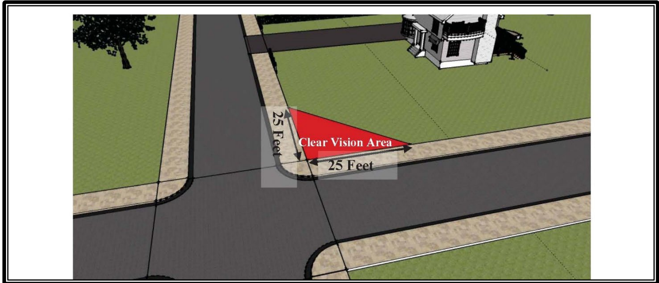
Figure VII-58 Clear Vision Area-Street Intersection
