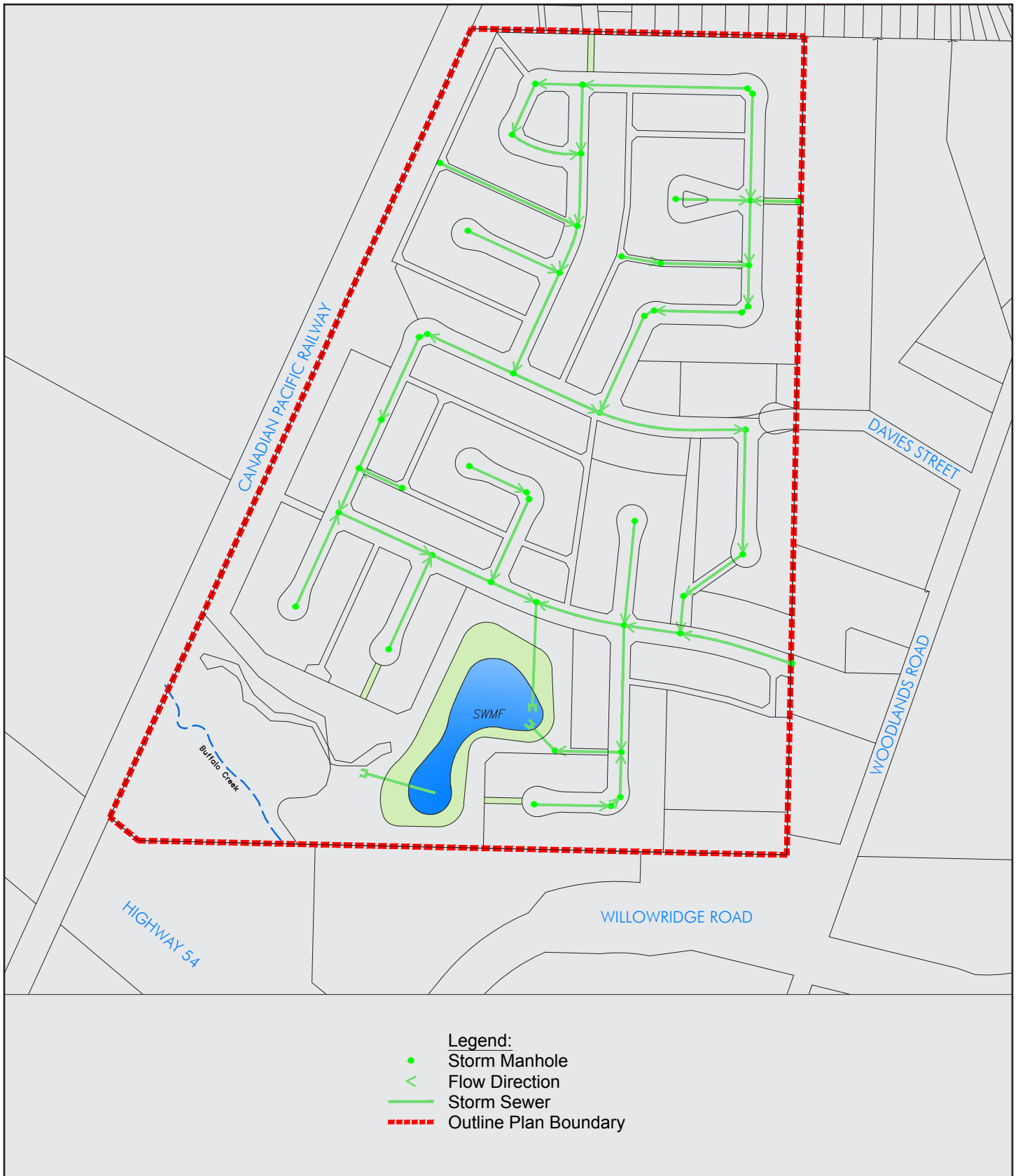
Figure 4 - Storm Sewer The Woodlands May 2014
