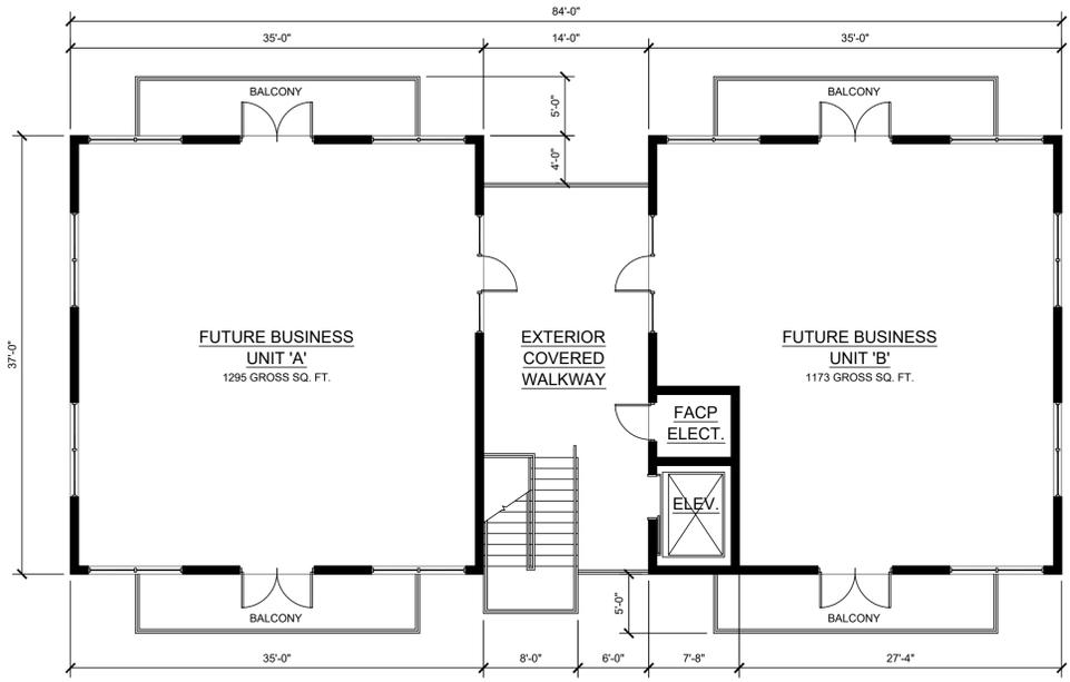
**SCHEMATIC SECOND FLOOR PLAN**
