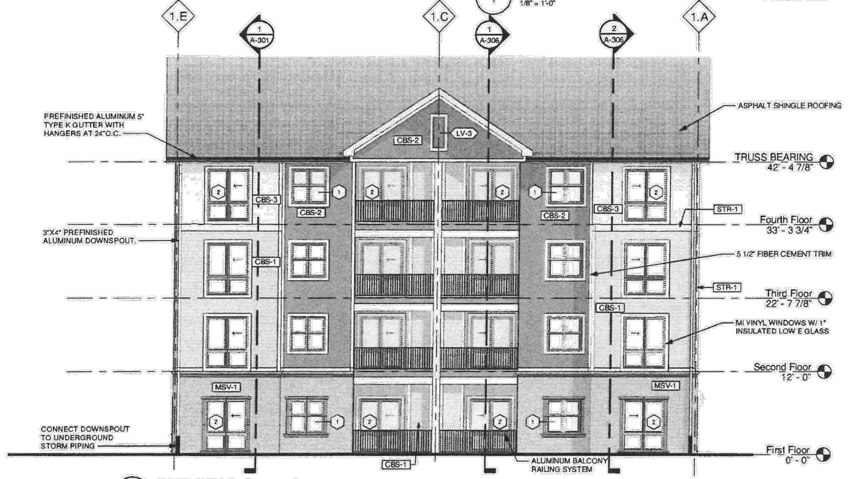
BUILDING 1 - WEST ELEVATION 1/8" = 1'-0"
