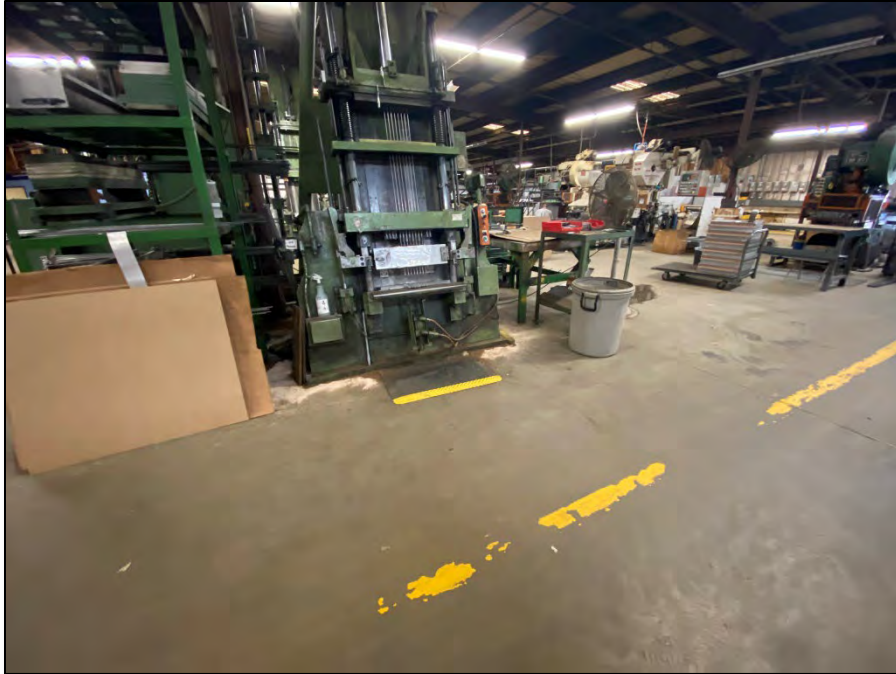
Photo 5. View of shop interior. Drawing fluid and/or hydraulic oil leaks are controlled beneath manufacturing equipment using oil-absorbent pads or granular absorbent.
