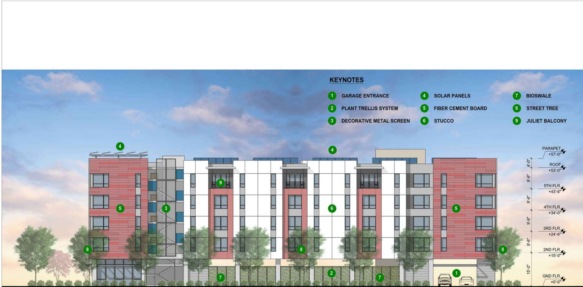
SOUTH ELEVATION - ALONG ALAMEDA DE LAS PULGAS
