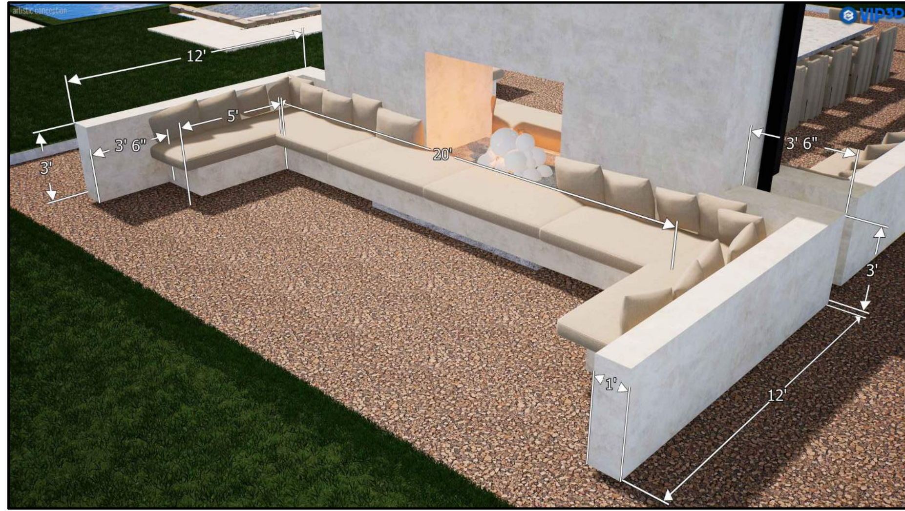
G Built In Place Seating at Dining Area NTS Construction Legend Reference SA-11
