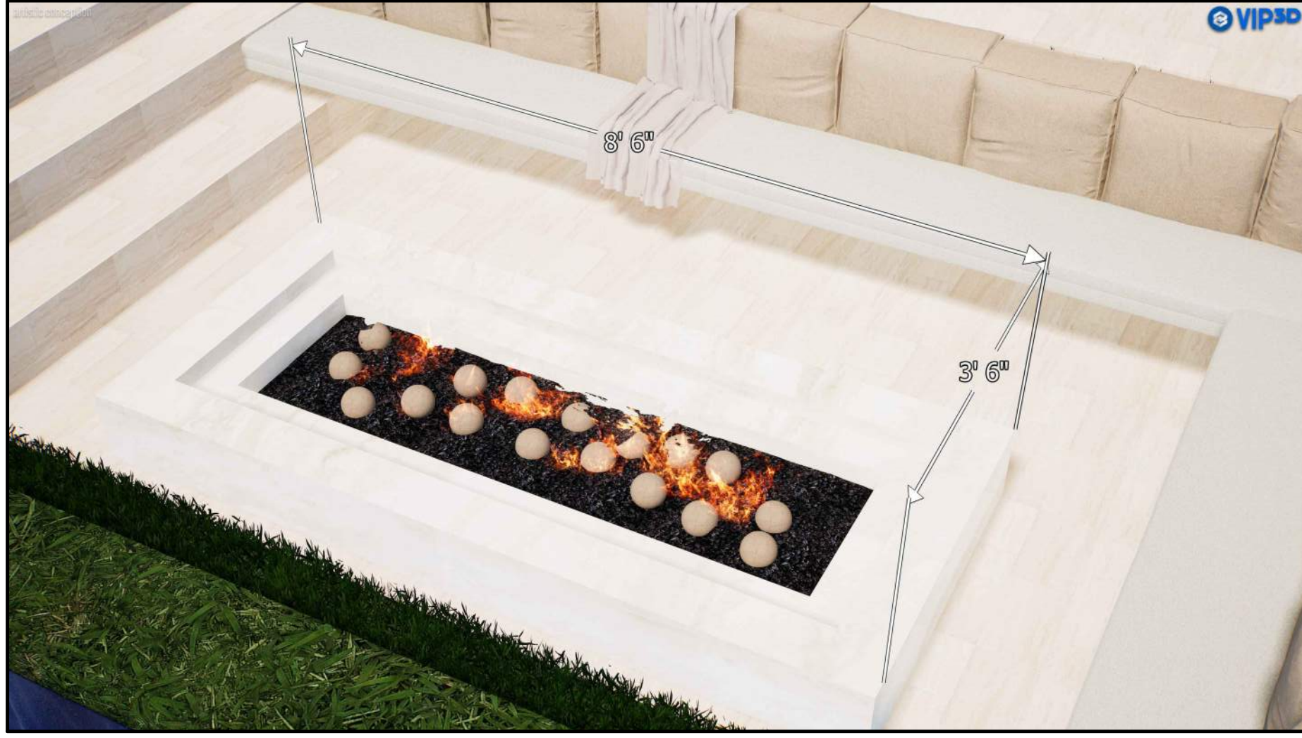
H 18"H Custom Fire Pit at Rectilinear Sunken Area NTS Construction Legend Reference SA-19
