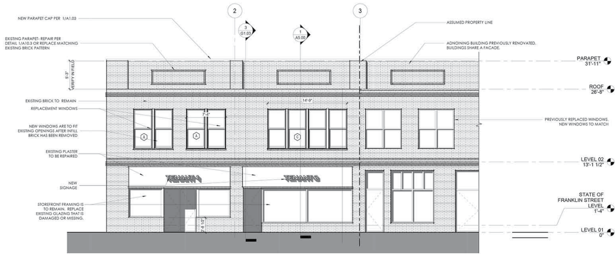
1 SPRING STREET EXISTING ELEVATION AFTER RENOVATION 3/16" = 1'-0"
