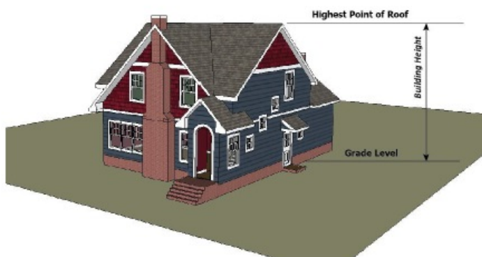
Figure 154.04-J: Measurement of building or structure height
