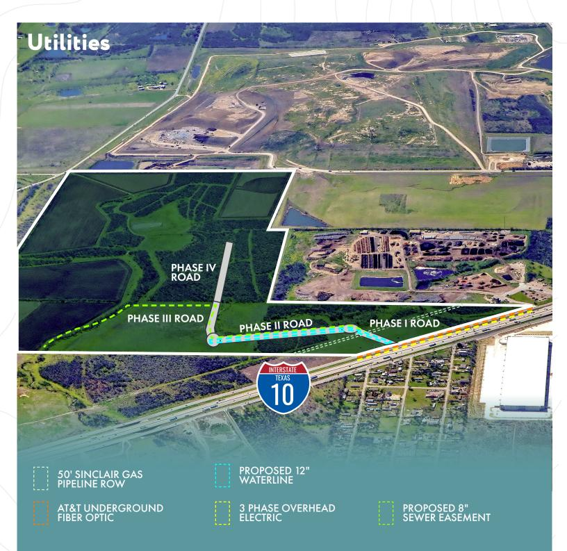
**10 East Industrial Park** is planned to be developed with fully entitled sites with all utilities. The site will include a new public road, built in up to four phases with water and sewer lines running along road. The proposed road is a four-lane road with turning access to accommodate large trucks.
