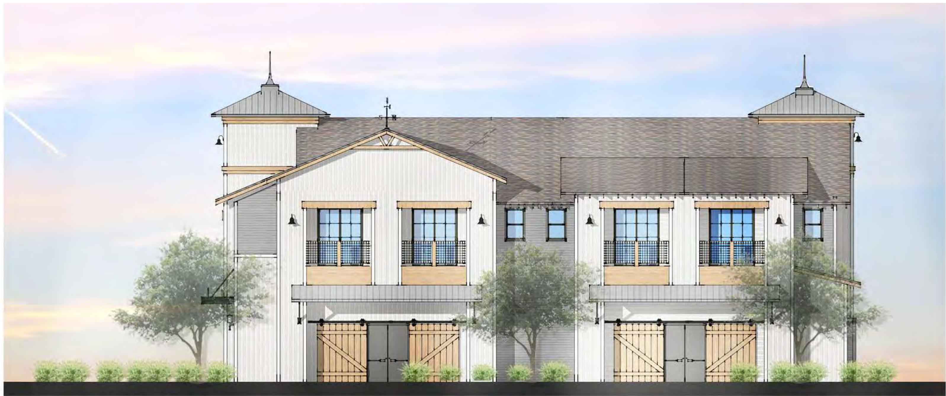
3 EAST ELEVATION-COMMERCIAL BUILDING 1/8" = 1'-0" (24 X 36 SHEET)
