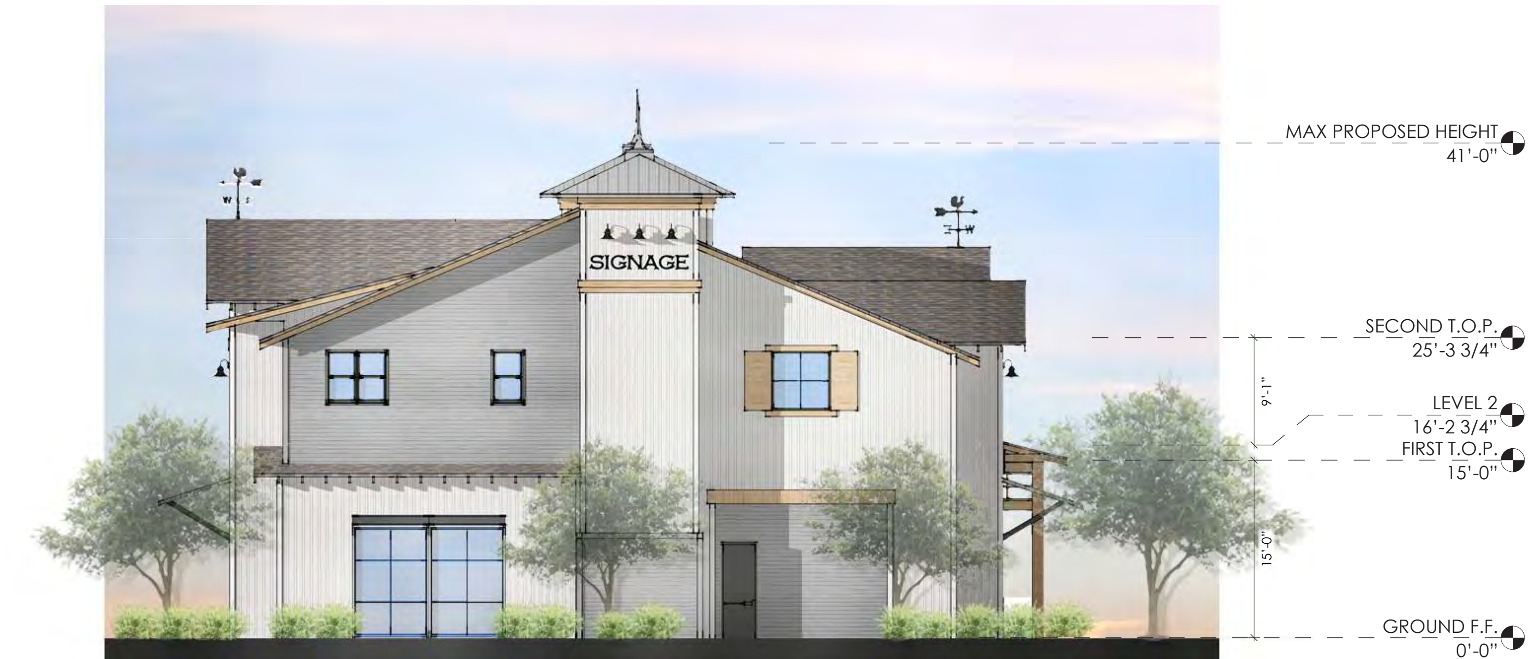
4 SOUTH ELEVATION-COMMERCIAL BUILDING 1/8" = 1'-0" (24 X 36 SHEET)
