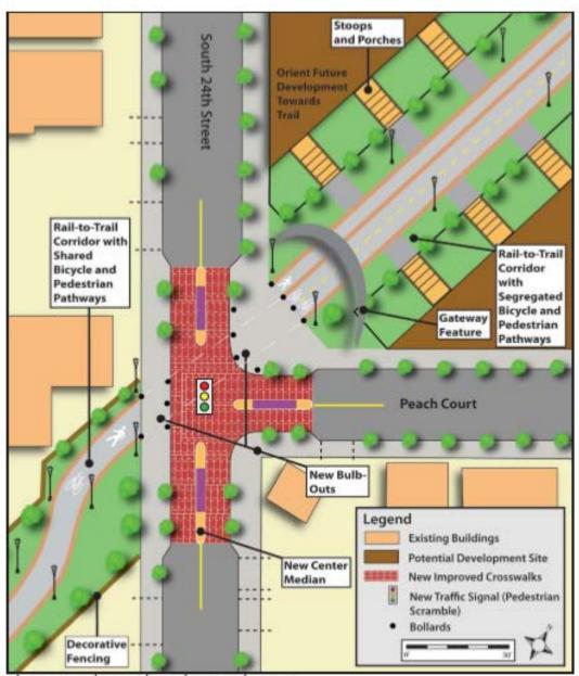
Figure 53. Rail-to-Trail corridor Detail Plan D.
