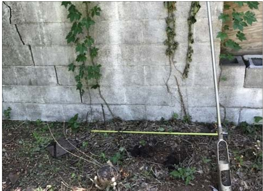
Photo 4: View of hand auger soil boring B-6 located on the western exterior wall of the garage
