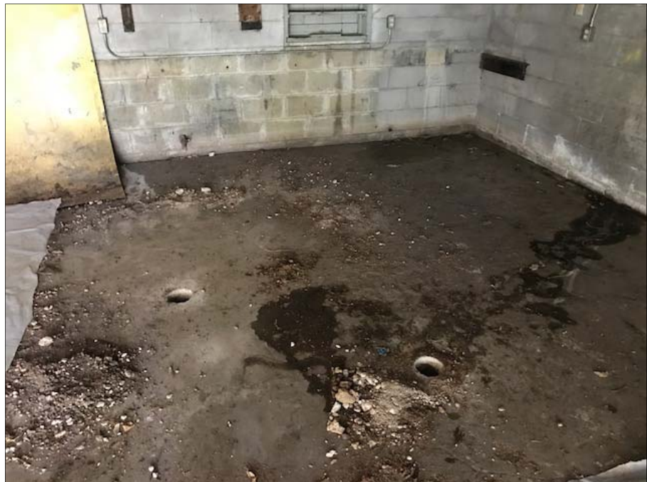
Photo 6: View of soil boring B-8 located on the interior of the garage, facing north. Note that the easternmost hole was abandoned due to refusal using a hand auger.
