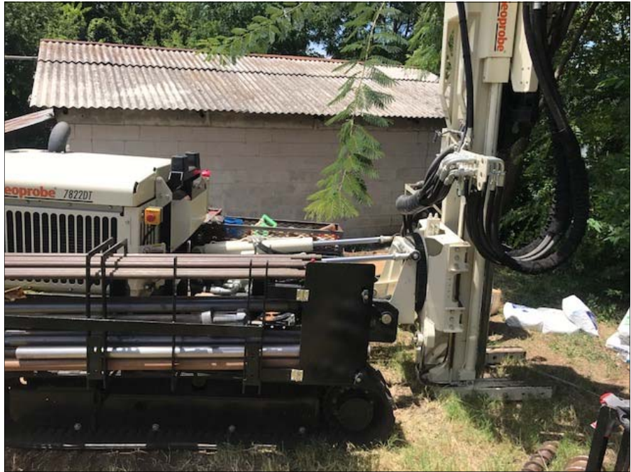
Photo 7: View of the advancement of soil boring B-9 located east of the garage, facing west.
