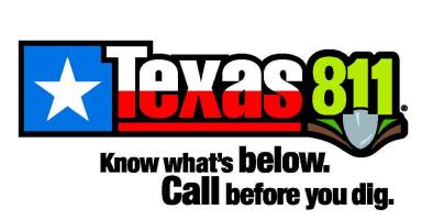
\*\*\* STOP! CALL BEFORE YOU DIG! \*\*\* AS REQUIRED BY "THE TEXAS UNDERGROUND FACILITY DAMAGE PREVENTION AND SAFETY ACT" TEXAS811 MUST BE CONTACTED AT LEAST 2 WORKING DAYS PRIOR TO ANY EXCAVATION OPERATIONS BEING PERFORMED. IT IS THE CONTRACTOR'S RESPONSIBILITY TO CONTACT TEXAS ONE CALL SYSTEM.
