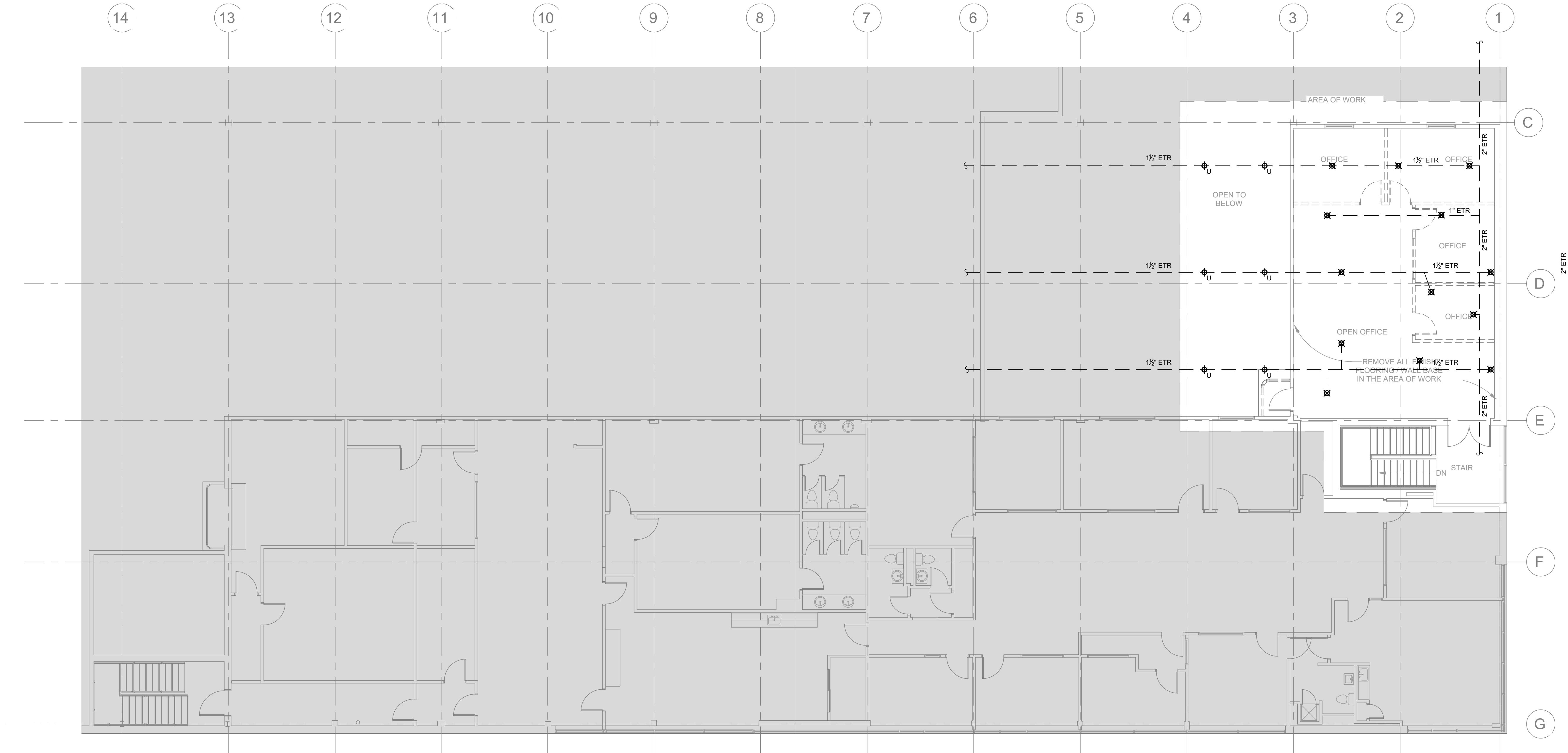
1 FIRE PROTECTION MEZZANINE DEMOLITION PLAN SCALE: 1/8" = 1'-0"
